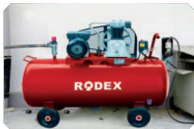
Faster cooling and less noise thanks to the pulley system
